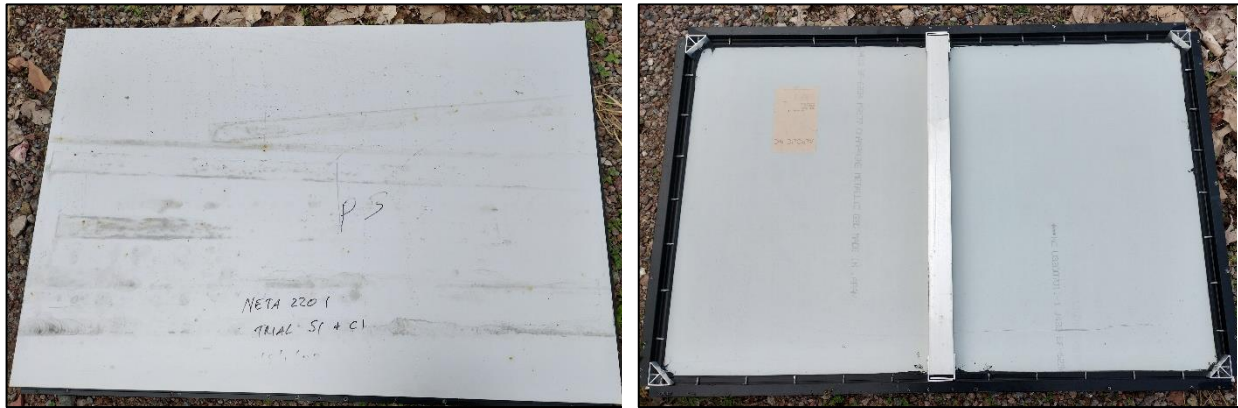
Figure 1: Photograph of Mitsubishi ALPOLIC NC cladding profile (note the 1,200 by 800 mm panel is displayed, larger panels have additional stiffeners)
