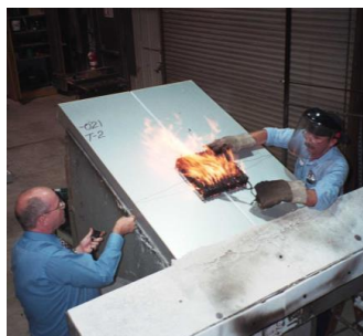
Example of fire test for roof
