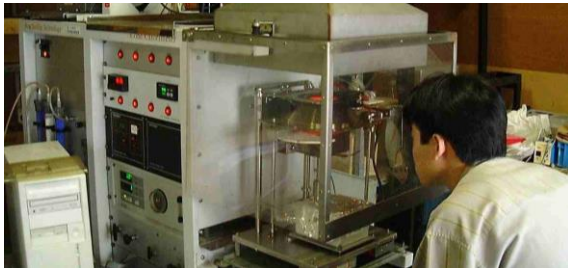
Fig. 2-8 Fire test in Japan, ISO 5660-1
