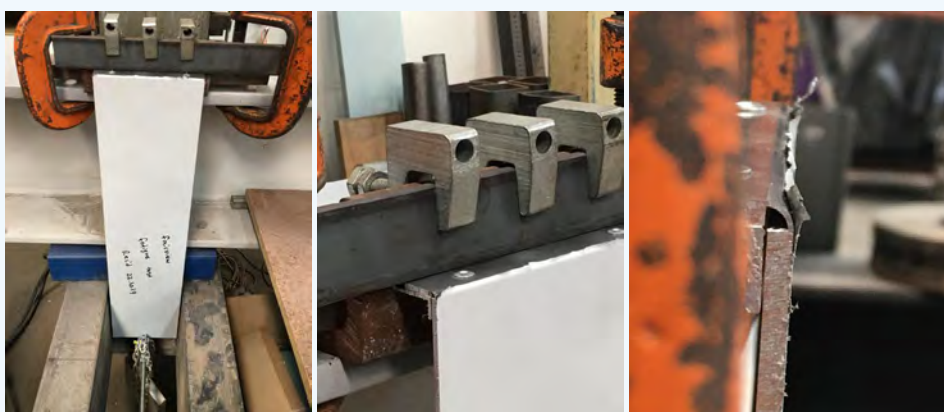
Figure 16.8: Fatigue testing of solid aluminium panels
