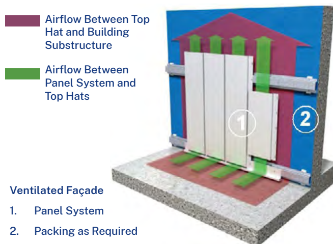
Figure 16.2: Ventilated façade principles (airflow)
