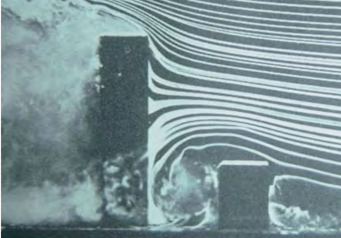
Figure 14.2: Wind Load Effects of Surrounding Buildings - downwash is augmented by upwind shorter building (after Penwarden and Wise, 1975)
