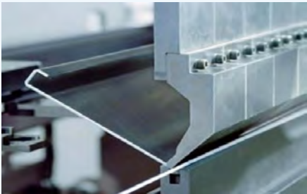
Figure 16.4: Folding of aluminium sheet using mechanical methods including break pressing
