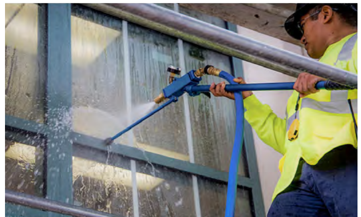
Figure 5.7: Window hose testing
