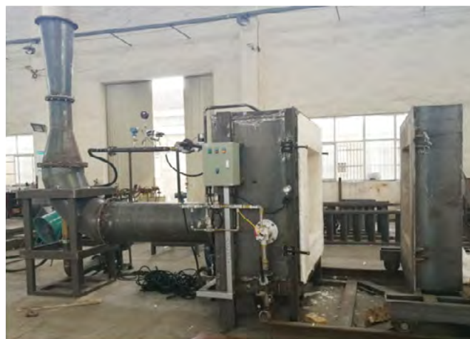
Figure 10.3: AS 1530.4 Testing Rig
