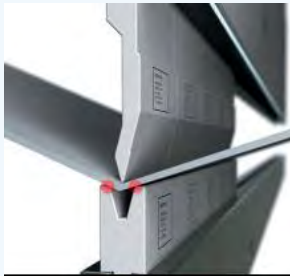
Figure 16.4: Folding of aluminium sheet using mechanical methods including break pressing
