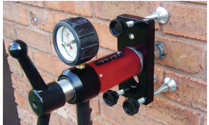
Figure 5.6: Masonry pull-out test
