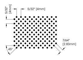
Hole diameter: Open area: Max. width of perforation: Max. plate width: 1/16" [1.5mm] 22.00% 4'-8 11/16" [1440mm] 4'-7 1/8" [1400mm]
