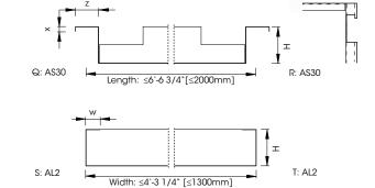
AS 30: H= 1 3/16" [30mm] | z= 9/16" [14mm] | x= 3/16" [5mm] AL 2: H= 1 9/16"[40mm] | w= 15/32" [12mm]
