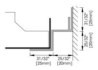
F 2025 shadow gap wall angle For lay-on perimeter panels
