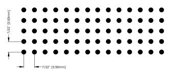
Hole diameter: Open area: Max. width of perforation: Max. plate width: 3/32" [2.5mm] 16.20% 4'-8 3/4" [1441mm] 4'-7 1/8" [1400mm]
