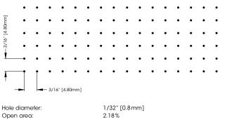
Open area: Max. width of perforation: Max. plate width: 1/32" [0.8mm] 2.18% 4`-2 1/16" [1 272mm] 4`-7 1/8" [1 400mm]
