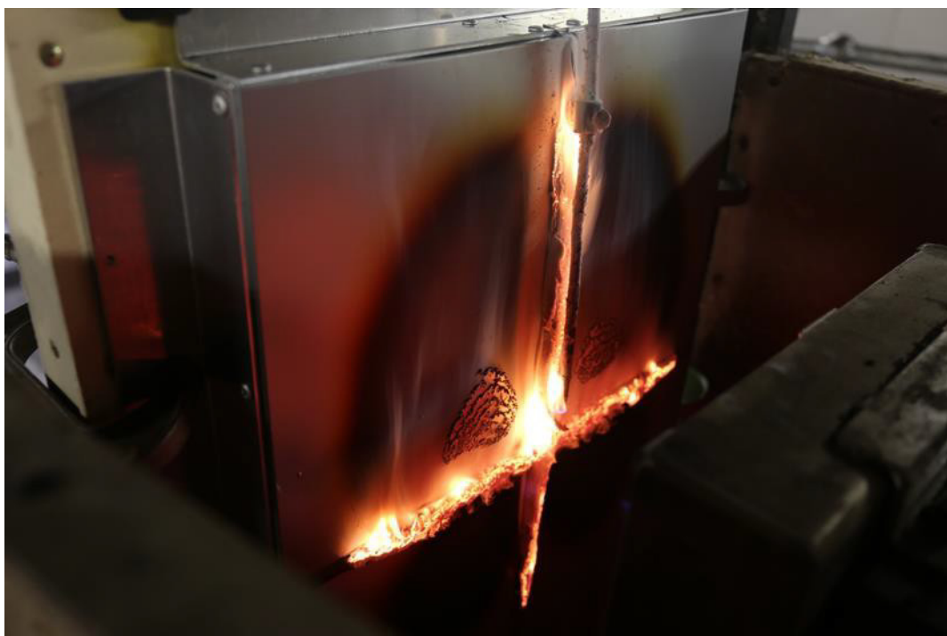
Figure 8 Aluminium composite panel test sample, ignition
