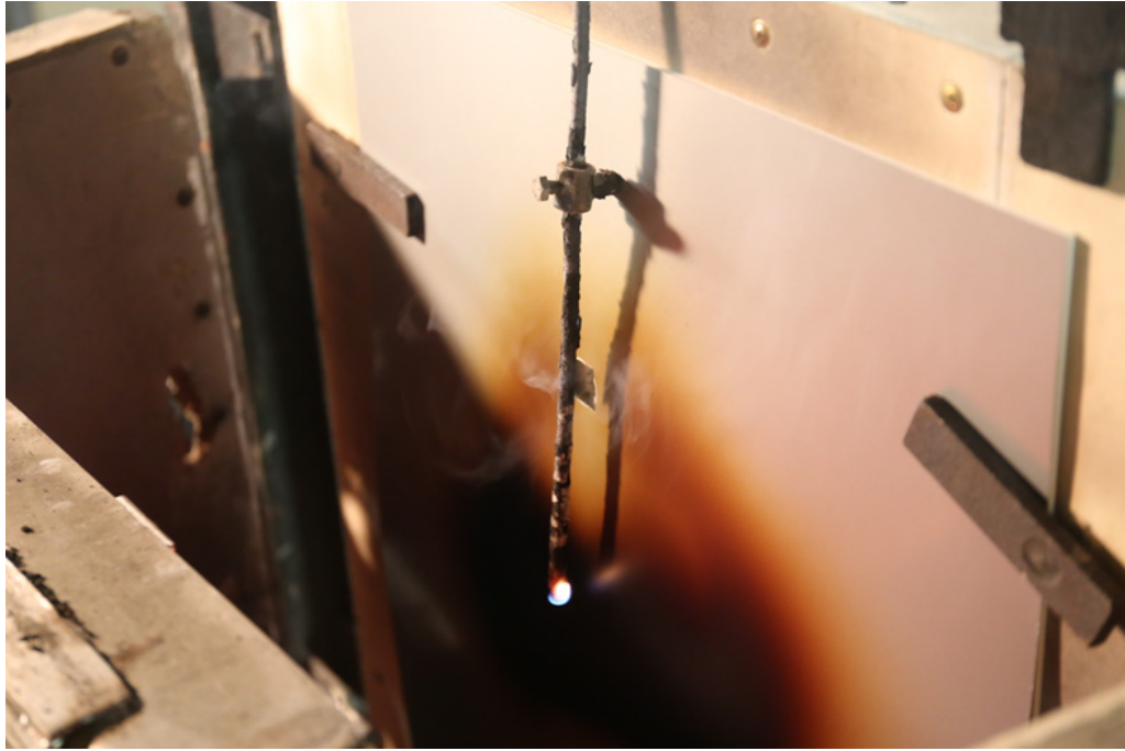
Figure 2 Aluminium composite panel test sample, ignition
