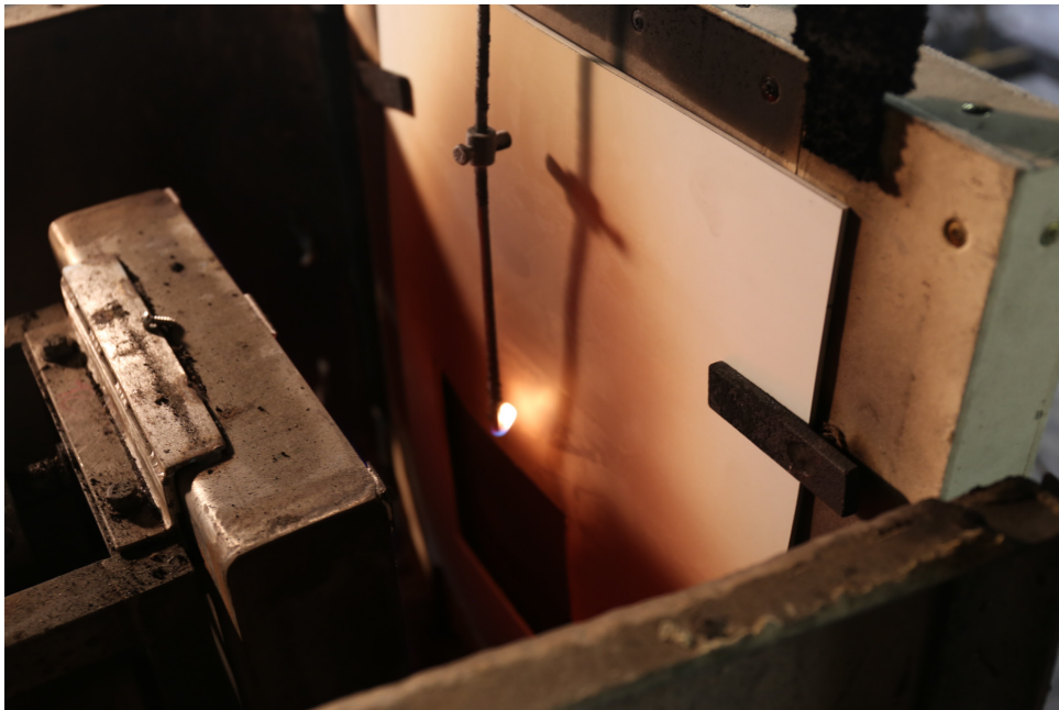
Figure 14 Aluminium composite panel test sample, ignition
