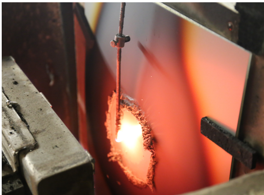
Figure 20 Aluminium composite panel test sample, ignition
