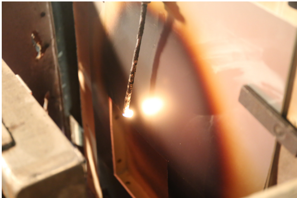
Figure 5 Aluminium composite panel test sample, ignition
