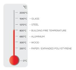
Thermometer showing aluminium melting and ignition points
